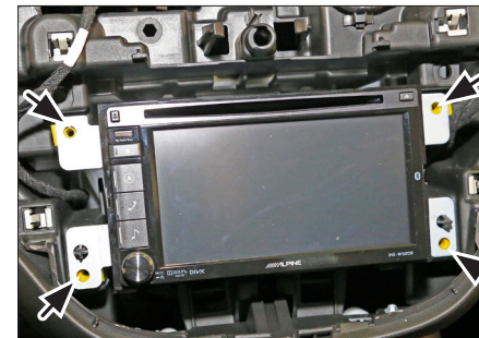
8. Connect all required circuit points Place Double DIN head unit on dash board
