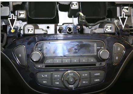
4. Remove 2 screws of head unit cover
