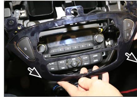
6. Remove OEM cover (unplug all connectors carefully)
