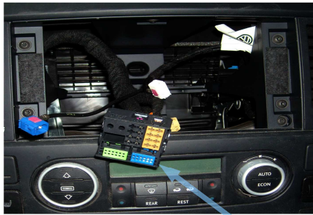
CAN-Abgriff am orig. Radiostecker Tap CAN on the orig. headunit connector
