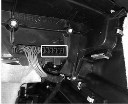
9. Connect the 8-Way connector to the MOST Interface
