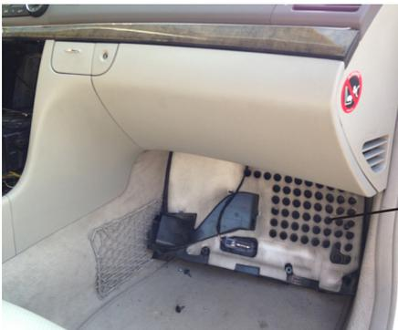
Remove panel to gain access to CAN Hub
