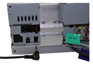
4. Connect the 14 way molex connector to the interface.
